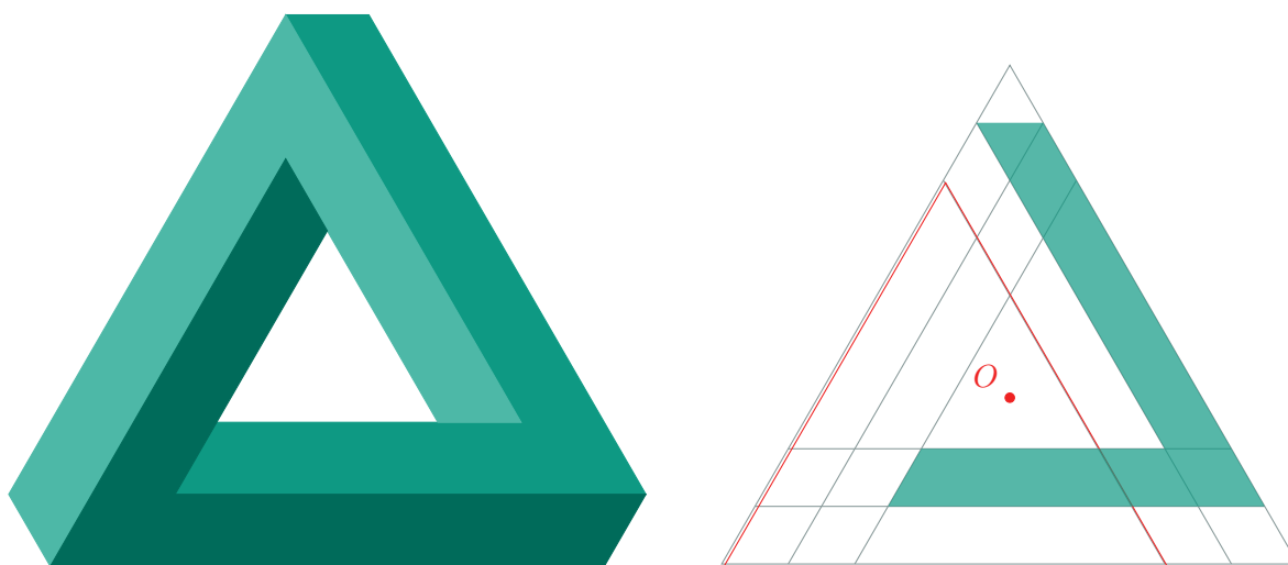
Figure 42: The construction of the Penrose triangle: the triangle is constructed by performing on the turquoise element (the right drawing), two rotations of 60 and 120 degrees respectively, centered at O . The red triangle can be seen as the building brick of the whole figure.
