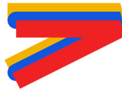
Figure 4: The three possibilities for line cap distinguished by colors, rect , round , butt
